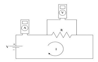
2. Switch on the power supply. Measure the current through and voltage across the resistor for 11 values of input voltage, in one volt increments, ranging from 2 V through 12V. Make a table for your voltage and current values associated with this resistor to include in your lab report.
