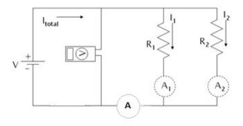
8. Switch on the power supply and adjust the voltage to 6 V. Record the total current and voltage values. Again, it's wise to use the Extech meter to validate this voltage.
