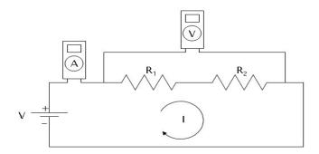
4. Switch the power supply on and adjust the voltage to 6 V. Record the current and voltage values as measured by your multimeters.
